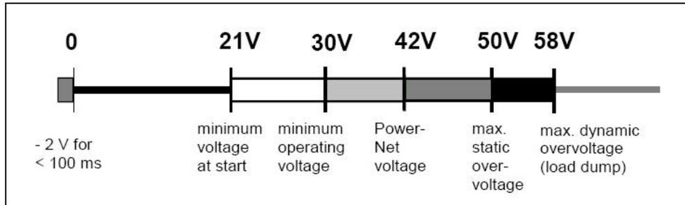
**Figure 1.2. Power net voltage requirements for 42V (Traub, 1999).**
