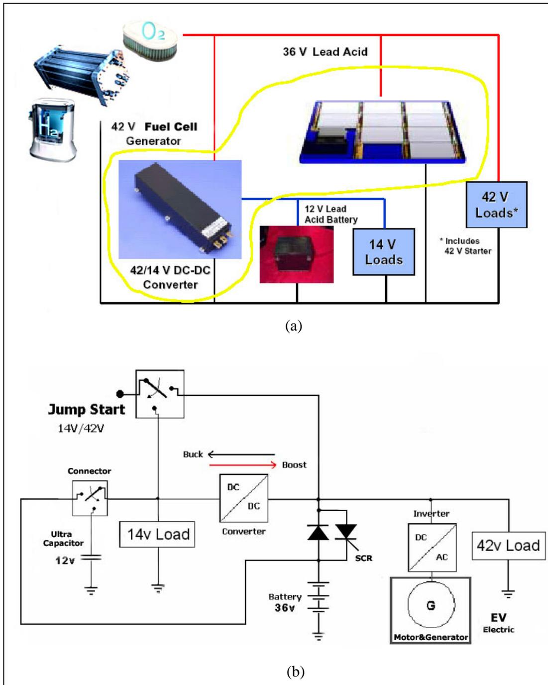
**Figure 1.4. (a) Basic block diagram of 42V EV electrical architecture system. (b) Block circuit diagram of 42V EV system with jump start post. The bidirectional converter handles the power transition of the two different bus system 14V and 42V. The main source of power comes from the 12V ultra capacitor, 36V battery and the 42V generator (Traub, 1999).**
