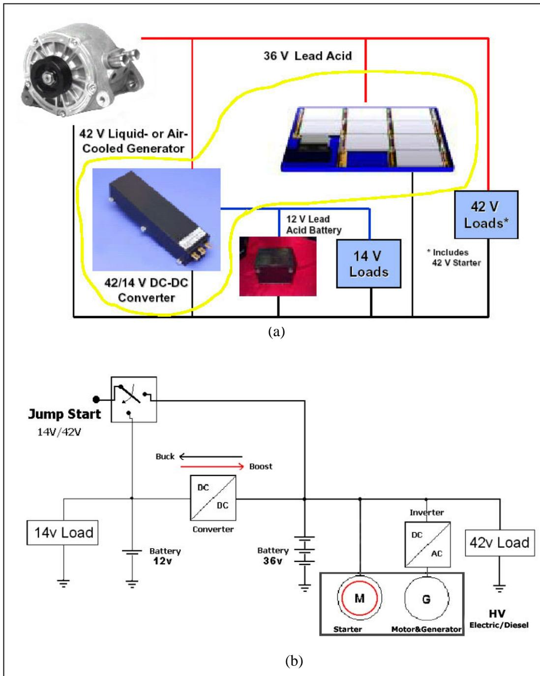
Figure 1.3. (a) Basic block diagram of 42V HV electrical architecture system. (b) Block circuit diagram of 42V HV system with jump start post. The bidirectional converter handles the power transition of the two different bus system 14V and 42V. The main source of power comes from the 12V battery, 36V battery and the 42V generator (Traub, 1999).
