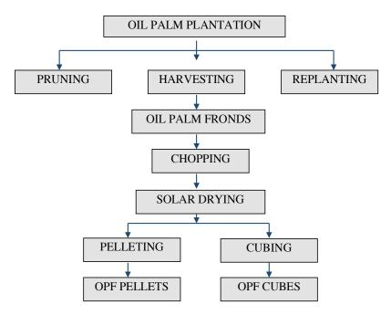
*Figure 4.* Schematic representation of the process of making OPF pellet and cube (adapted from Mat Daham et al., 2002)
