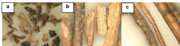
Figure 7 Observation of OPEFB particle geometry; spherical shape (a), flake-like (b), and cylinder-like (c), after treated with 210°C of superheated treatment
