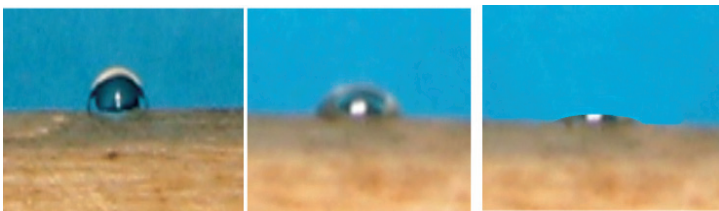
Figure 19 Wetting of kenaf core surface - A water droplet after 30 sec.(left); 1 min. (centre) and 5 min. (right). Source: Paridah et al. (2009)
