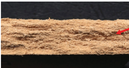
Lack of adhesion in MDF made from empty fruit bunch (EFB) fibres caused by low surface wetting (Norul Izani et al. , 2013).
