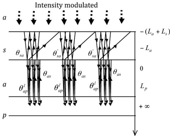
**Figure 3** One-dimensional configuration of photopyroelectric cell with the route of thermal wave showed; s is sample, a is air, p is PVDF film, b is backing. (Azmi et al, 2006)
