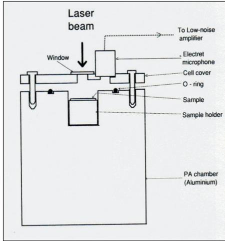
**Figure 5** The small volume PA cell
