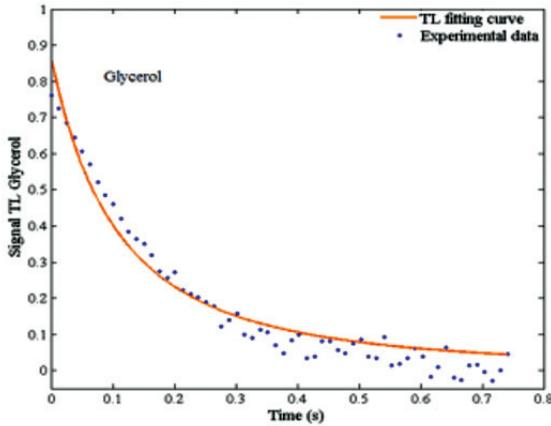
**Figure 27** The thermal lens signal obtained by pulsed excitation.
