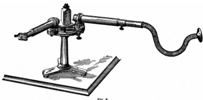
**Figure 1** Bell's instrument for observing the photothermal effect. ([http://fys.kuleuven.be/atf/Research\\_themes/rt\\_photoacoustic/rt\\_photo pha](http://fys.kuleuven.be/atf/Research_themes/rt_photoacoustic/rt_photo pha))
