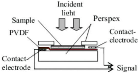
**Figure 6** Schematic diagram of sample-PVDF holder
