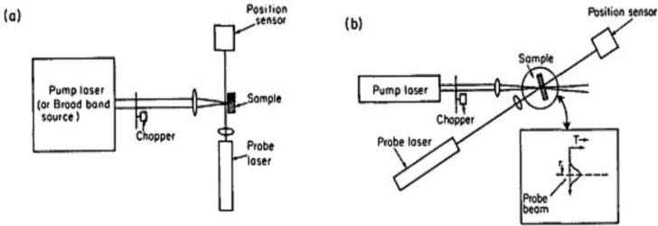
**Figure 8** Photothermal Beam Deflection method (a) transverse, (b) collinear. (Jackson et al, 1980)
