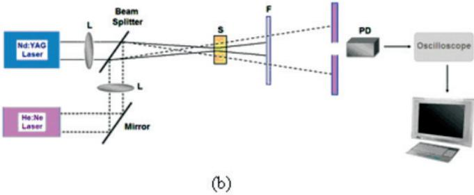
**Figure 7** Schematic diagram of Thermal lens experimental set up using (a) CW excitation beam (Reza et al, 2011), (b) pulsed excitation beam. (L = lens, S = sample; F = filter; PD = photodiode detector) (Reza et al, 2012).
