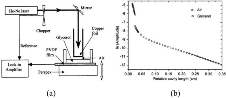
**Figure 23** (a) Schematic diagram of the experimental setup. (b) The amplitude of the pyroelectric signal on the cavity length for the two layer fluids: air and glycerol. The solid lines are the best-fit results of the experimental data. (Azmi et al., 2005)
