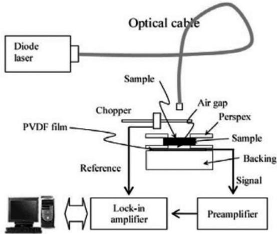
**Figure 24** Measurement of thermal diffusivity using Non-Contact pyroelectric method. (Azmi et al, 2006)
