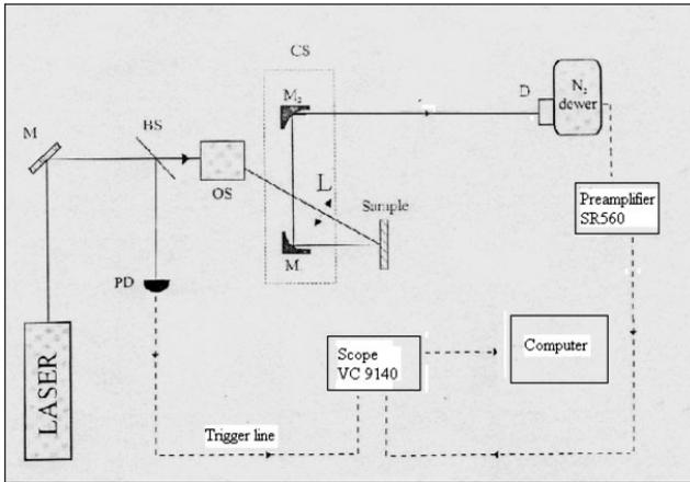
**Figure 11** Schematic diagram of transient heat detection. D=CdHgTe detector, BS = beam splitter, OS = optical system, PD = photodetector, CS = signal collection system. (Moksin et al, 1999).
