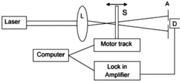
**Figure 9** Z-scans setup. L = lens, S = sample, A = aperture, D = detector. (Shahriari et al, 2010)
