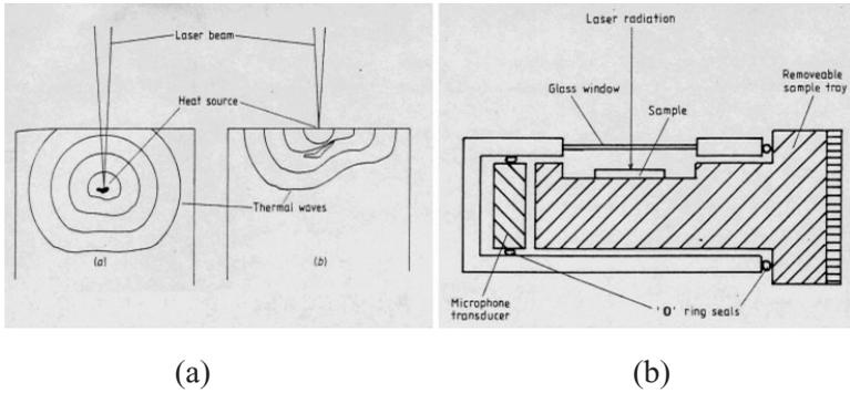
**Figure 13** (a) The generation of imaging information by the interaction of thermal waves with physical structures for transparent and opaque samples, (b) Schematic diagram of a photoacoustic gas cell. (Kirkbright et al, 1984)
