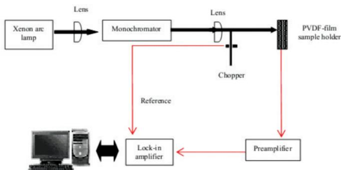
**Figure 12** Schematic diagram of photopyroelectric spectrometer. (Azmi et al., 2004)
