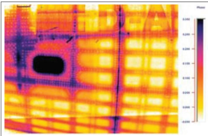
**Figure 19** Fuselage inspection of a Boeing 737 using lock-in thermography shows the skin lap joints, stringers, doublers, and rivets. This image shows no defects. The frame station and the frame window appear in a darker color, an indication that they are made out of thicker material. (Vision Systems Design)
