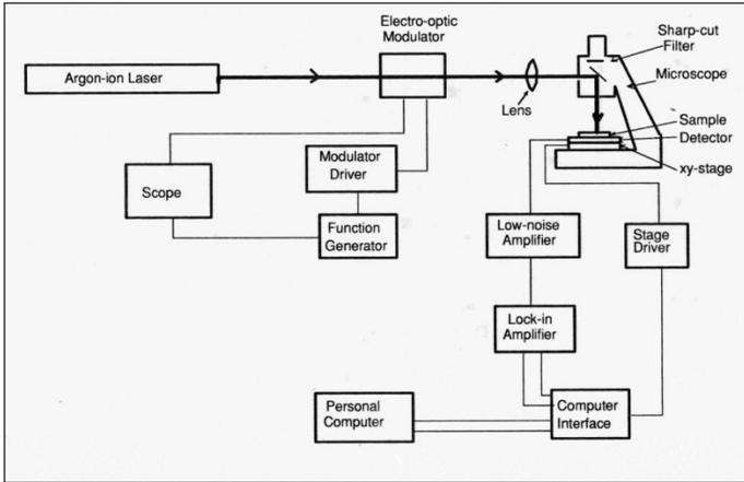
**Figure 15** Scanning photothermal microscopy system
