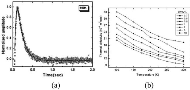
**Figure 26** (a) The transient signal by PVDF detector at the back of sample after photoflashing (b) The thermal diffusivity curves of sample at various temperature. (Moksin et al, 2013)
