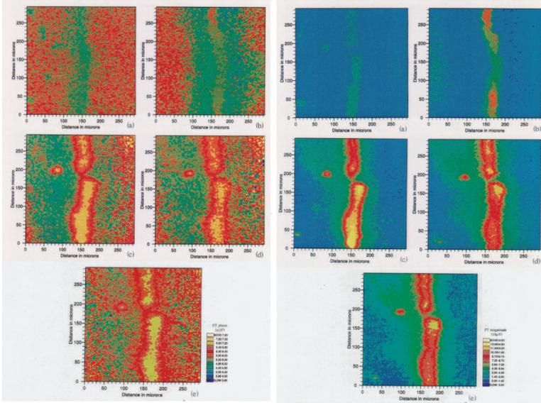
(A) PZT phase images of a deliberately scratched gold-coated Kapton sample scanned at 2 kHz: (a) unexposed, (b) exposed to a fluence of  $24.6 \times 10^{20}$  atom/cm<sup>2</sup>. The phase images of the last exposure sample exposed to a fluence of  $28.3 \times 10^{20}$  atom/cm<sup>2</sup> and scanned at different light chopping frequencies (c) 2.0 kHz, (d) 1.3 kHz, (e) 0.9 kHz.
