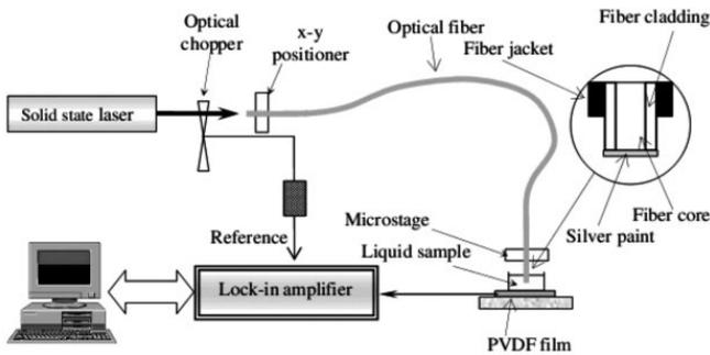
**Figure 25** Schematic diagram of FO-TWRC technique.
