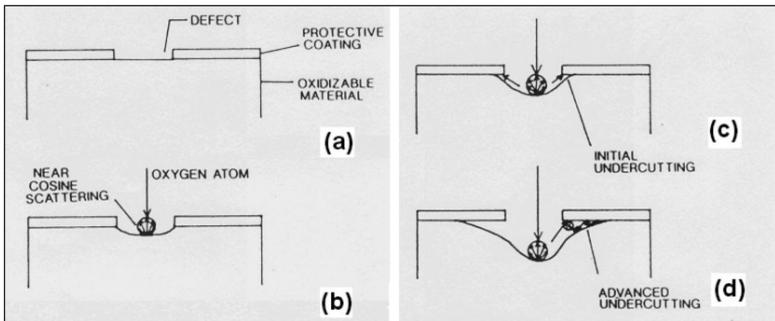
**Figure 16** A possible scenario for undercutting of a defect coating in an ATOX environment. (Banks and Rutledge, 1988)
