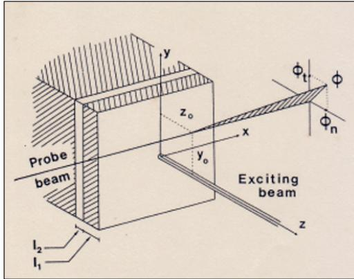
**Figure 10** Geometry employed in mirage detection of semi-infinite slab. (Salazar et al., 1991)
