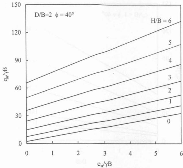
Fig. 9(b): Variation of  $q_u/\gamma B$  with  $c_u/\gamma B$  at different values of  $H/B$  at  $\phi = 40^\circ$  and  $D/B = 2$
