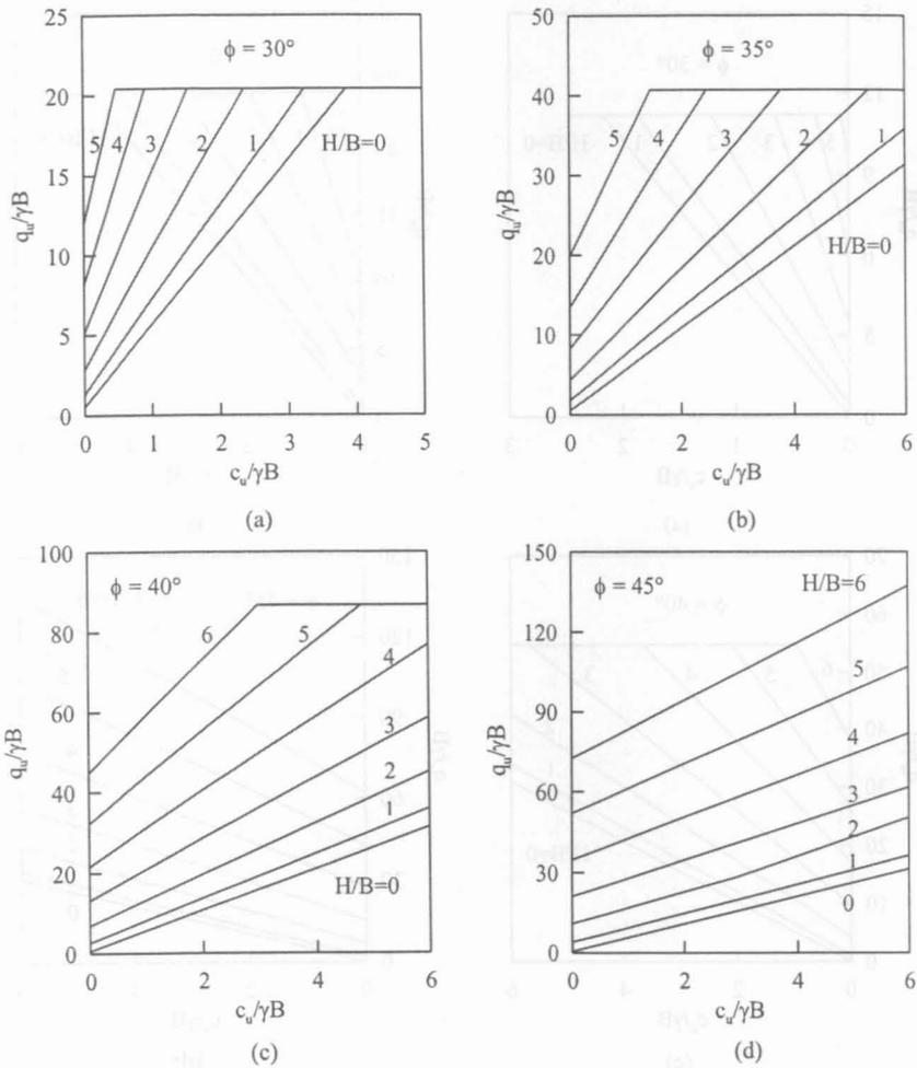
Fig. 12: Variation of  $q_u/\gamma B$  with  $c_u/\gamma B$  for sand-clay foundation soil at  $D/B = 0.5$ : (a)  $\phi = 30^\circ$ , (b)  $\phi = 35^\circ$ , (c)  $\phi = 40^\circ$  and (d)  $\phi = 45^\circ$
