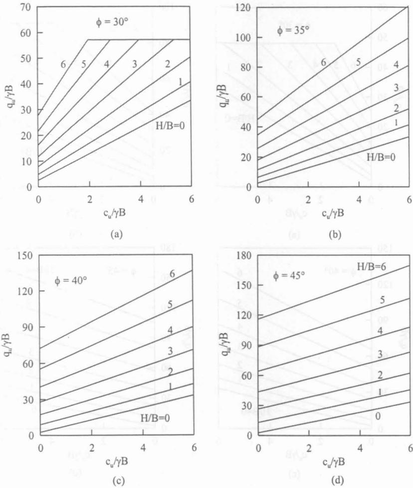
Fig. 16: Variation of  $q_u/\gamma B$  with  $c_u/\gamma B$  for sand-clay foundation soil at  $D/B = 2.5$ : (a)  $\phi = 30^\circ$ , (b)  $\phi = 35^\circ$ , (c)  $\phi = 40^\circ$  and (d)  $\phi = 45^\circ$
