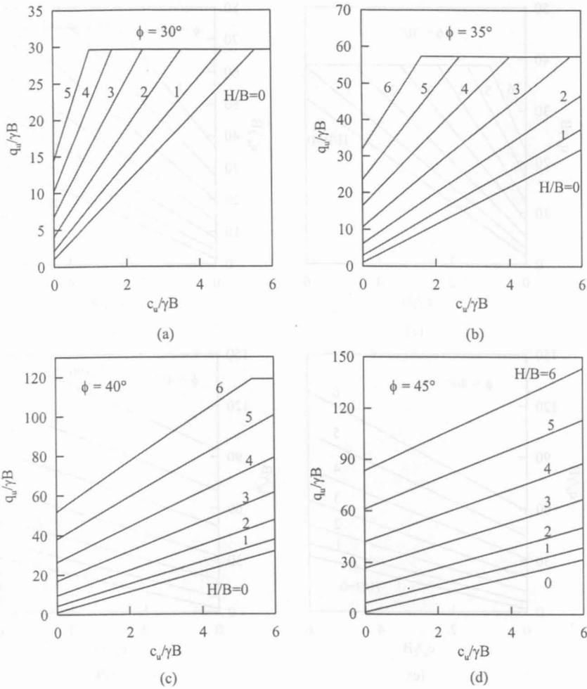
Fig. 13: Variation of  $q_u/\gamma B$  with  $c_u/\gamma B$  for sand-clay foundation soil at  $D/B = 1.0$ : (a)  $\phi = 30^\circ$ , (b)  $\phi = 35^\circ$ , (c)  $\phi = 40^\circ$  and (d)  $\phi = 45^\circ$
