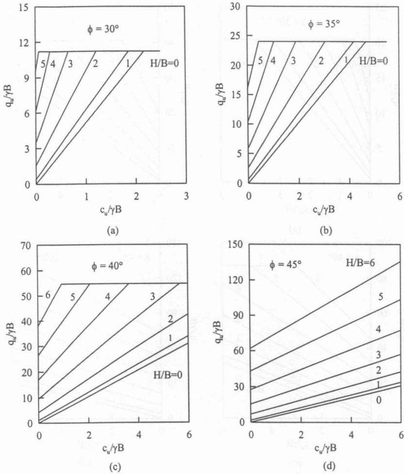
Fig. 11: Variation of  $q_u/\gamma B$  with  $c_u/\gamma B$  for sand-clay foundation soil at  $D/B = 0$ : (a)  $\phi = 30^\circ$ , (b)  $\phi = 35^\circ$ , (c)  $\phi = 40^\circ$  and (d)  $\phi = 45^\circ$
