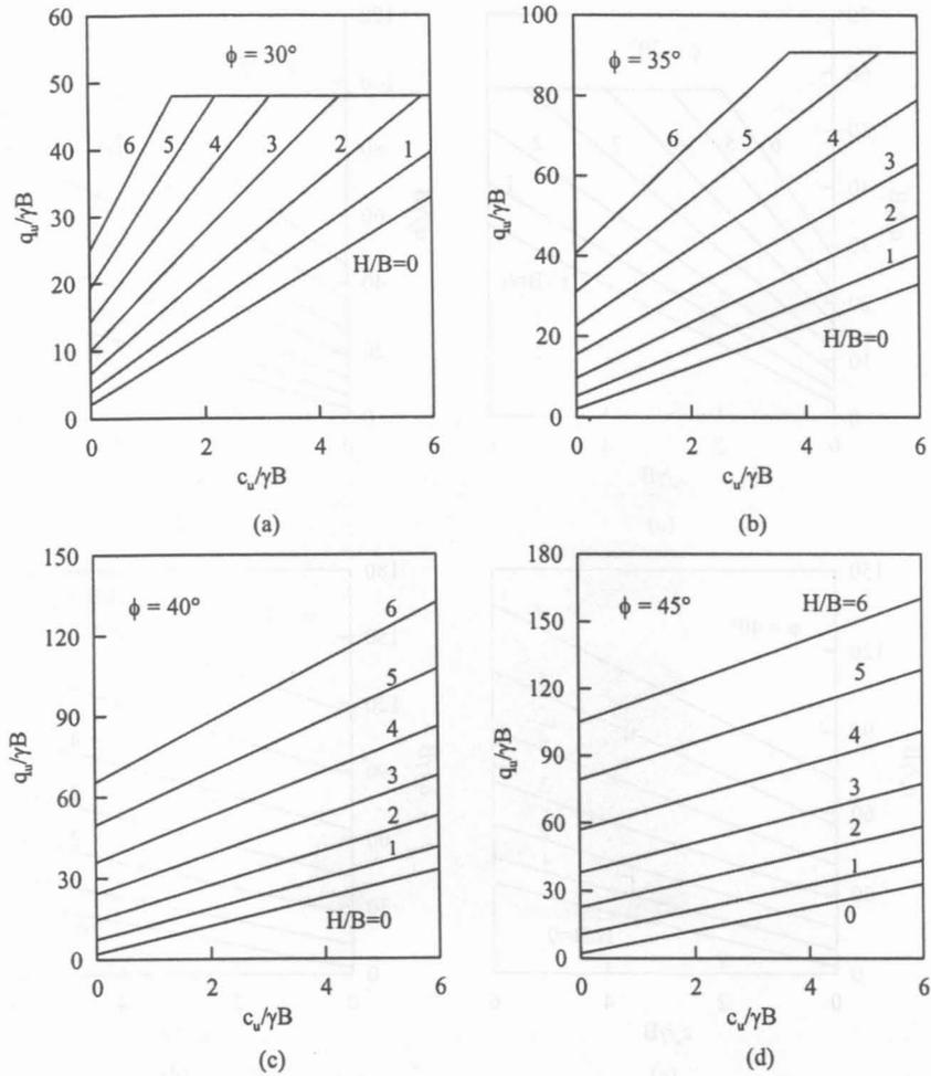
Fig. 15: Variation of  $q_u/\gamma B$  with  $c_u/\gamma B$  for sand-clay foundation soil at  $D/B = 2.0$ : (a)  $\phi = 30^\circ$ , (b)  $\phi = 35^\circ$ , (c)  $\phi = 40^\circ$  and (d)  $\phi = 45^\circ$
