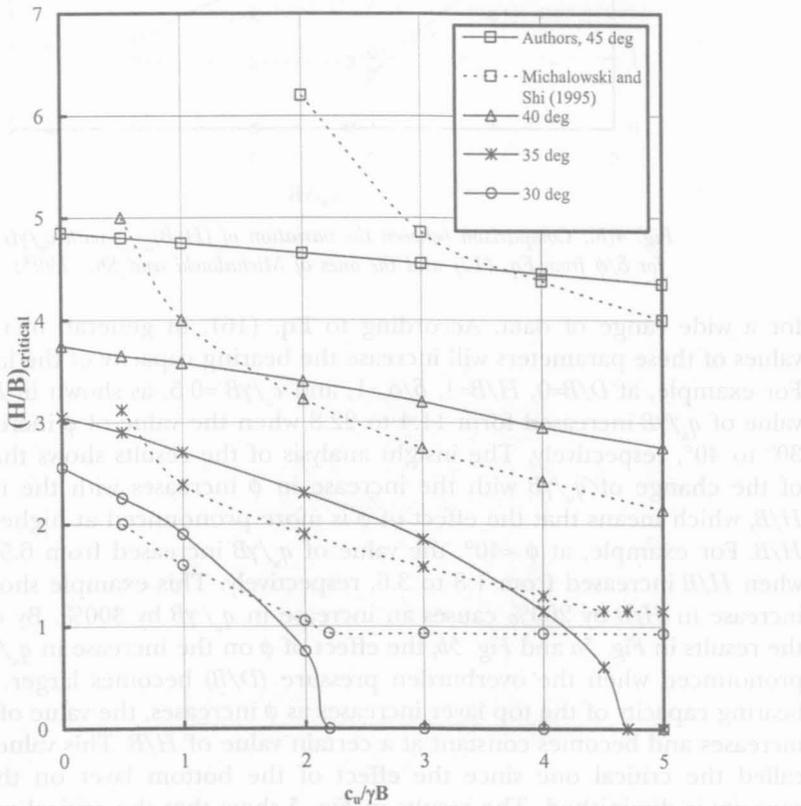
Fig. 4(a): Comparison between the variation of  $(H/B)_{critical}$  with  $c_u/\gamma B$  for  $\delta/\phi = 1.0$  and the ones of Michalowski and Shi (1995)
