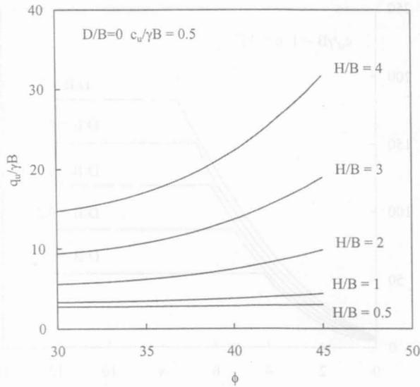
Fig. 6(a): Effect of  $H/B$  on the variation of  $q_u/\gamma B$  with angle of friction ( $\phi$ ) at  $D/B = 0$  and  $c_u/\gamma B = 0.5$
