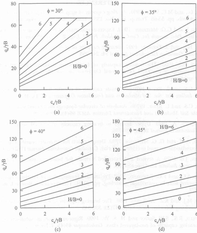
Fig. 17: Variation of  $q_u/\gamma B$  with  $c_u/\gamma B$  for sand-clay foundation soil at  $D/B = 3.0$ : (a)  $\phi = 30^\circ$ , (b)  $\phi = 35^\circ$ , (c)  $\phi = 40^\circ$  and (d)  $\phi = 45^\circ$
