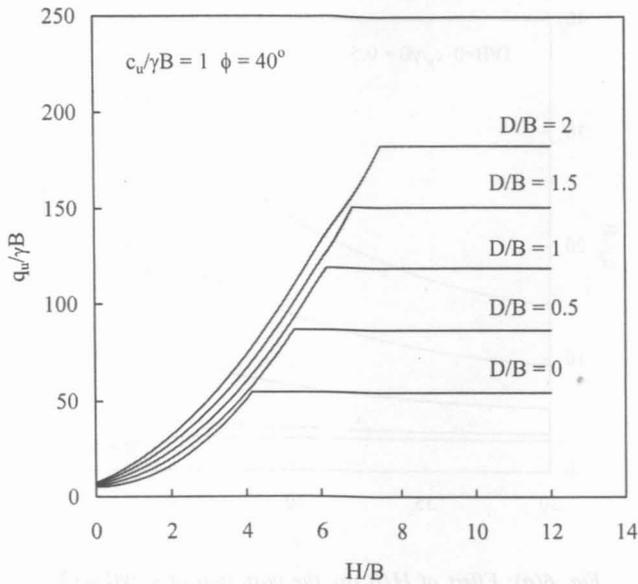
Fig. 7: Effect of D/B on the variation of  $q_u/\gamma B$  with H/B at  $f = 40^\circ$  and  $c_u/\gamma B = 1$
