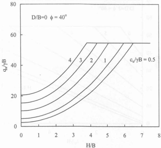
Fig. 10: Variation of  $q_u/\gamma B$  with  $c_u/\gamma B$  at different values of  $H/B$  at  $\phi = 40^\circ$  and  $D/B = 2$
