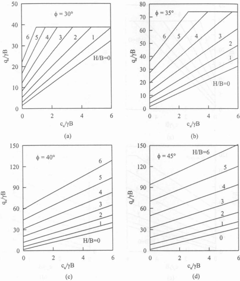
Fig. 14: Variation of  $q_u/\gamma B$  with  $c_u/\gamma B$  for sand-clay foundation soil at  $D/B = 1.5$ : (a)  $\phi = 30^\circ$ , (b)  $\phi = 35^\circ$ , (c)  $\phi = 40^\circ$  and (d)  $\phi = 45^\circ$
