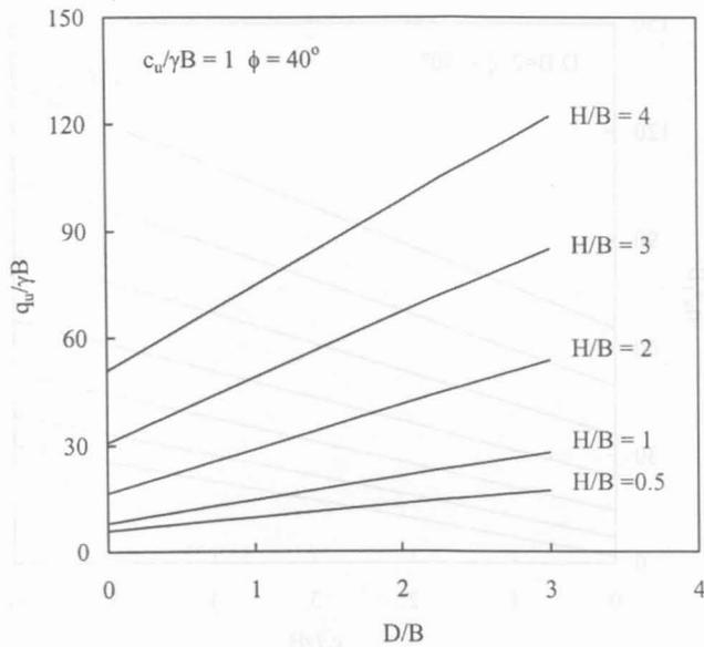
Fig. 8: Variation of  $q_u/gB$  with  $D/B$  at different values of  $H/B$  at  $\phi = 40^\circ$  and  $c_u/\gamma B = 1$
