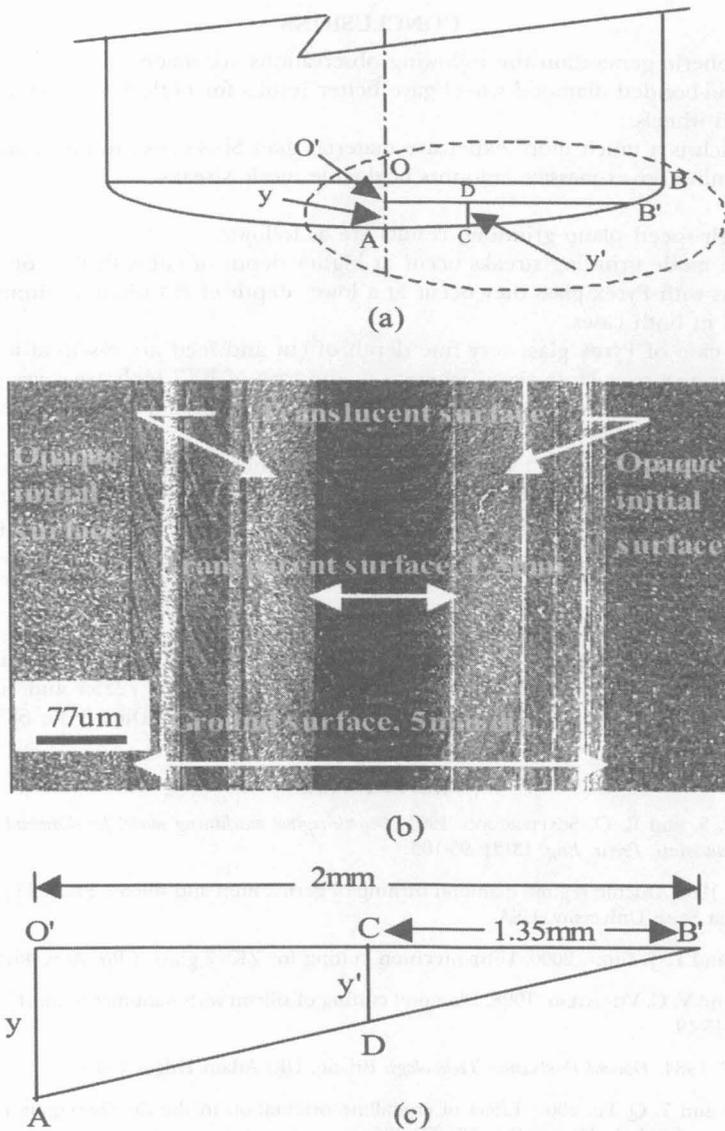
Fig. 11: (a) shows exaggerated conicity of grinding wheel (actual cone angle will be about  $179.4^\circ$ ). (b) Plan view of ground surface whose diameter is less than wheel diameter, because depth of cut is less than  $y$ . The central part despite being fractured is transparent and the outer part is translucent despite the partial ductile streaks. (c) Enlargement of triangular area  $O'BA$  in (a) for estimation of critical depth of cut ( $y'$ )
