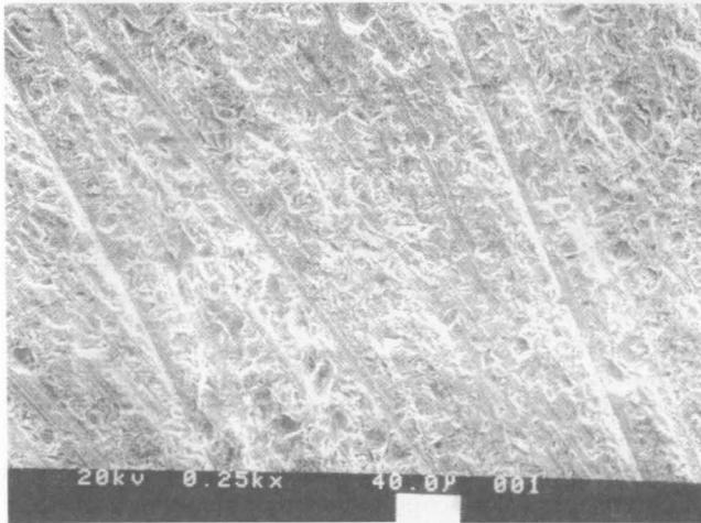
*Fig. 3: Ductile streaks obtained on Ge during aspheric generation*
