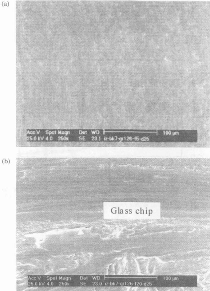
Fig. 10: SEM micrographs of ground BK7 glass surfaces are shown at depth of cut of 25 mm and feed of (a) 5 and (b) 20mm/min. Formation of a chip due to lateral ploughing action can be seen in (b).
