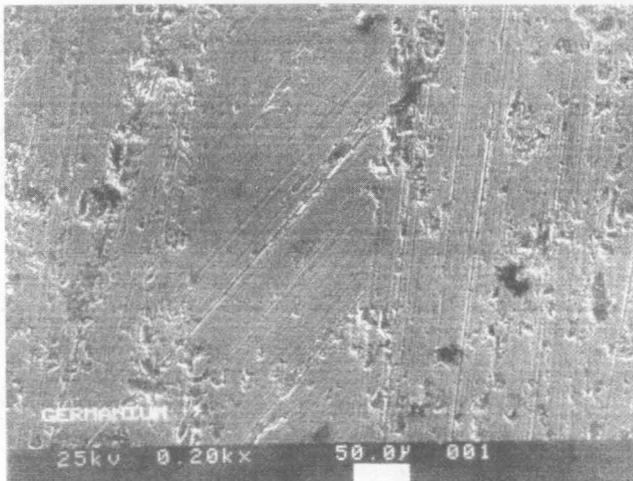
*Fig. 4: Massive formation of ductile streaks on Ge during aspheric generation with a resinoid-bonded diamond wheel*
