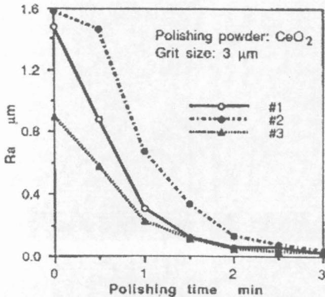
Fig. 8: Roughness value versus polishing time. Curve #1 with the largest amount of ductile streaks and maximum roughness achieved better surface finish faster than curve #3 which has the best surface finish (Venkatesh and Zhong 1995)
