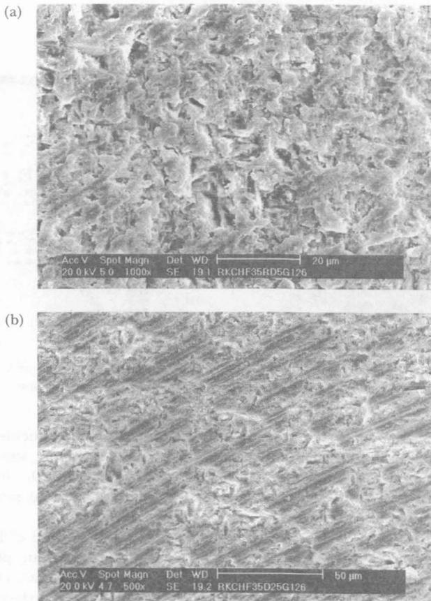
Fig. 6: SEM pictures of ground Si. The surfaces consist of (a) microfractures and (b) grinding streaks
