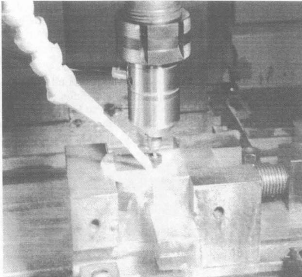
Fig. 2: High speed jig grinding of silicon and glass
