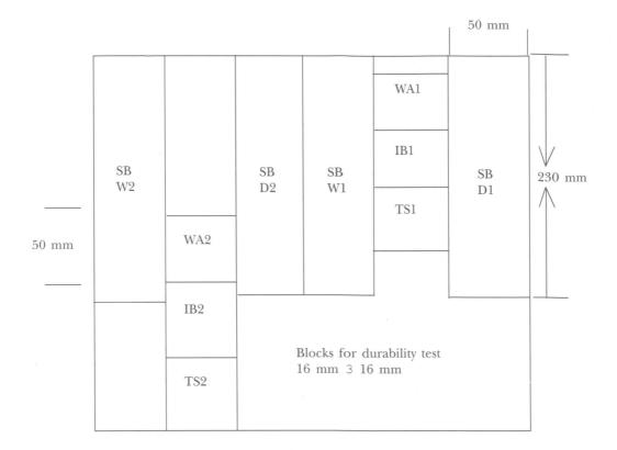
SBW = Wet static bending sample SBD = Dry static bending sample WA = Water absorption sample IB = Internal bond sample
