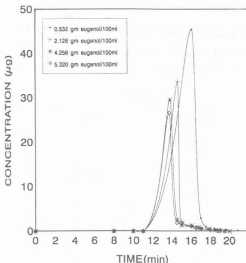
Fig 2. Chromatographic elution curves of eugenol on  $\mu$  Bondapak  $C_{18}$  analytical column, mobile phase methanol-water (80:20), flow rate 0.5 ml/min, at different solution concentration injection at equilibrium condition
