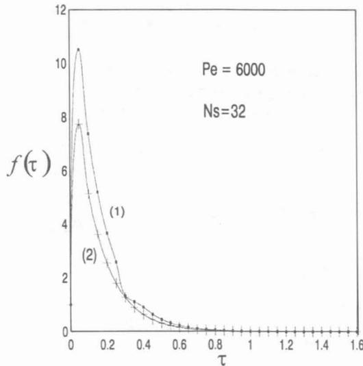
Fig 4. Theoretical chromatographic evolution curves of eugenol on  $\mu$  Bondapak  $C_{18}$  analytical column, mobile phase methanol-water (80:20), flow rate 0.7 ml/min, at different bed length parameters, (1)  $\delta=3.0$ , (2)  $\delta=0.3$
