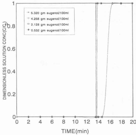
Fig 3. Experimental breakthrough curves at different eugenol injection concentration on  $\mu$  Bondapak  $C_{18}$  analytical column, mobile phase methanol-water (80:20), flow rate 0.5 ml/min
