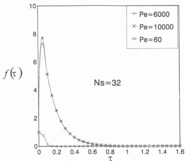
Fig 6. Theoretical chromatographic elution curve of eugenol on  $\mu$  Bondapak  $C_{18}$  analytical column, mobile phase methanol-water (80:20), flow rate 0.7 ml/min,  $\delta=0.3$ , at different Peclet number
