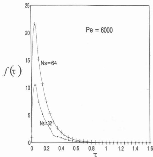
Fig 5. Theoretical chromatographic elution curve of eugenol on  $\mu$  Bondapak  $C_{18}$  analytical column, mobile phase methanol-water (80:20), flow rate 0.7 ml/min,  $\delta=0.3$ , at different sample points( $N_s$ )
