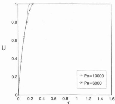
Fig 7. Theoretical breakthrough curve of eugenol on  $\mu$  Bondapak  $C_{18}$  analytical column, mobile phase methanol-water (80:20), flow rate 0.7 ml/min,  $\delta=0.3$ , at different Peclet number
