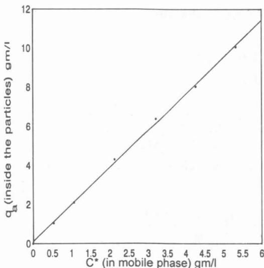
*Fig 1. Adsorption isotherm of eugenol at room temperature from packed bed equilibrium adsorption experiments on  $C_{18}$   $\mu$  Bondapak column (30 cm  $\times$  3.9 mm i.d.); mobile phase, methanol/water (80:20); flowrate, 0.5 ml/min.*
