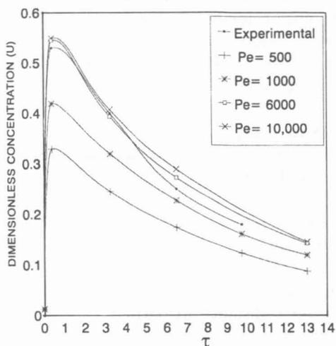
Fig 8. Experimental elution curve of eugenol superimposed on theoretical predictions elution curve at different Peclet numbers. (Experimental conditions  $\mu$  Bondapak  $C_{18}$  analytical column, mobile phase methanol-water [80:20], flow rate 0.7 ml/min. Simulation parameters  $\delta=3.0$ ,  $N_p=90$ )
