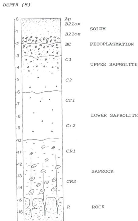
Fig. 1: A schematic sketch of a basalt profile
