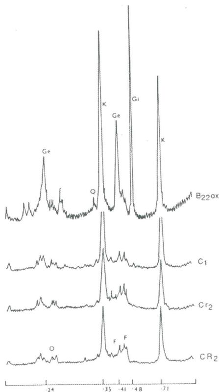
Fig. 3: The x-ray diffraction pattern of the Mg saturated clay size fraction of a basalt profile (Note: M-mica, Gi-gibbsite, Q-quartz, K-kaolinite, Ge-goethite)
