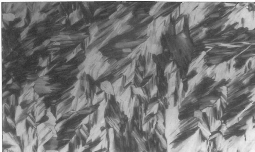
Plate 1. Optical pattern of typical hexagonal liquid crystalline structure at 50% by weight of both water and mixed surfactant
