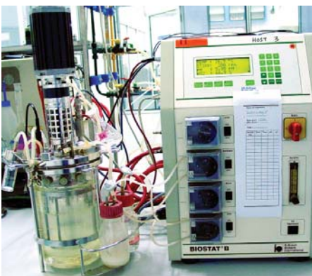
■ Stirred Tank Fermenter (2L) - Biostat B2
