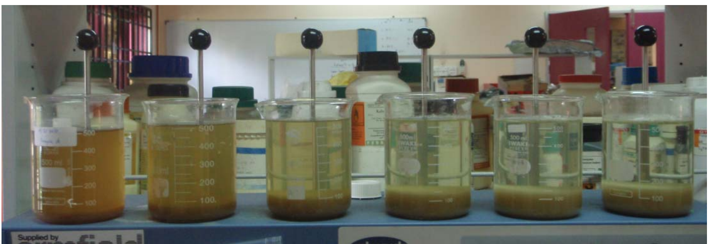
■ BOTTOM Final discharge treatment using alum with jar test equipment
