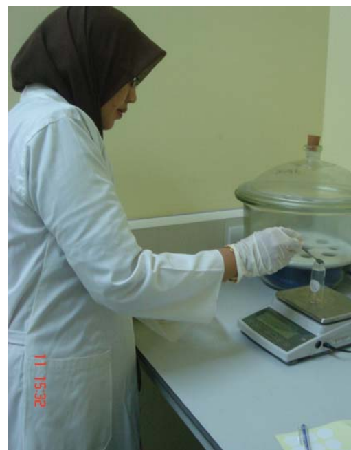
■ BOTTOM Weighing the ground OPEFB
