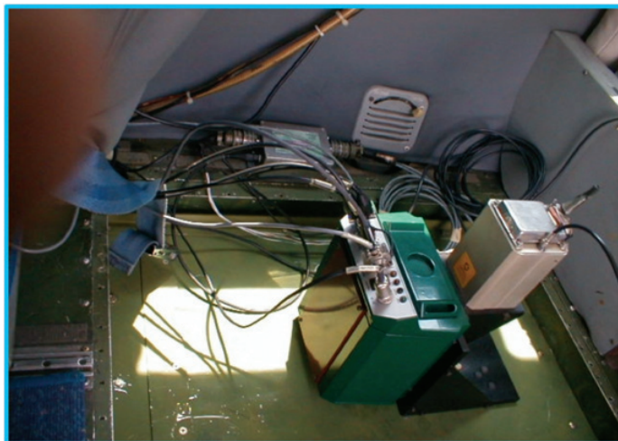
Figure 10 The close-up of the UPM-AISA classic mounted on an aluminum metal plate on-board a RMAF Cessna C402B aircraft
