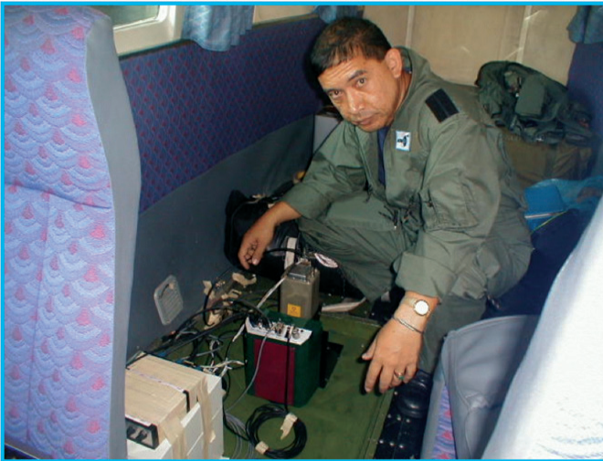
Figure 9 The UPM-AISA Classic mounting and installation on-board a RMAF Cessna C402B aircraft
