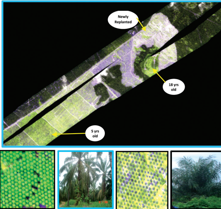
Figure 26 Oil palm plantation age map (above) with UPM-AISA sensor showing 18 years (bottom left) and 5 years old (bottom right) oil palm individual trees
