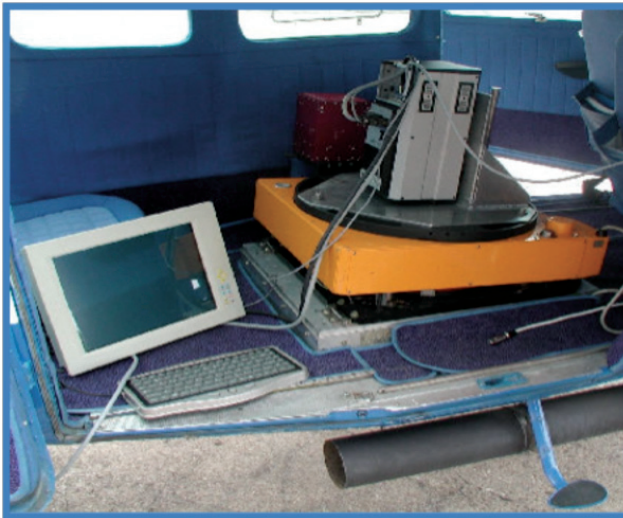
Figure 11 An AISA Eagle VNIR airborne hyperspectral system mounted in an aircraft
