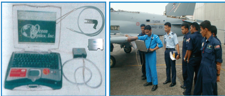
Figure 17 An ocean optic hand held spectroradiometer (left) being used to measure spectral signatures of a one-seater RMAF fighter jet that crashed into Mersing coast
