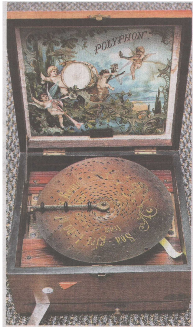
This is a J.H. Ebblewhite-made interchangeable disc music box dating back to the 1880s. It allowed owners to listen to different pieces by purchasing new discs like they would records.
