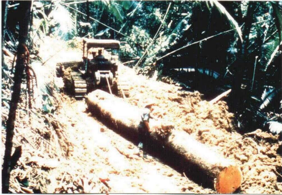
Plate 1. Extraction of Log Using Crawler Tractor on the Skid Trail.
